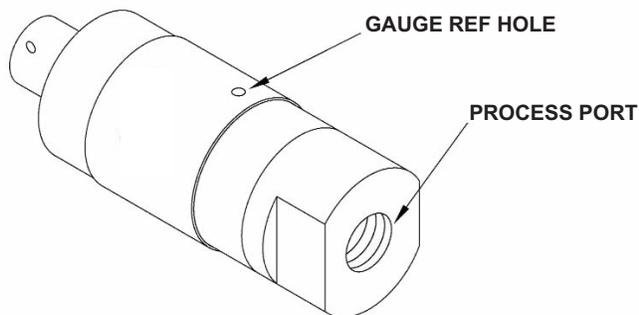
This vent hole insures both sides of the sensor are exposed to the local altitude and barometric pressure. This gauge reference hole equalizes these pressures and provides a stable zero reading regardless of barometric pressure or altitude. Therefore true gauge format provides a pressure measurement relative to local altitude and atmospheric conditions.
