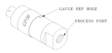
This vent hole insures both sides of the sensor are exposed to the local altitude and barometric pressure. This gauge reference hole equalizes these pressures and provides a stable zero reading regardless of barometric pressure or altitude. Therefore true gauge format provides a pressure measurement relative to local altitude and atmospheric conditions.
