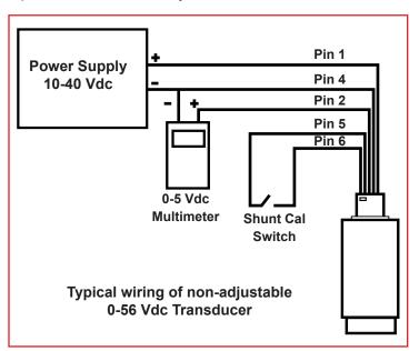
In order to operate these types of devices short or apply power to the appropriate pins. The pin-out can be found either on the performance certificate, marked on the transducers nameplate, our website or by contacting the factory with the model number or serial number.
